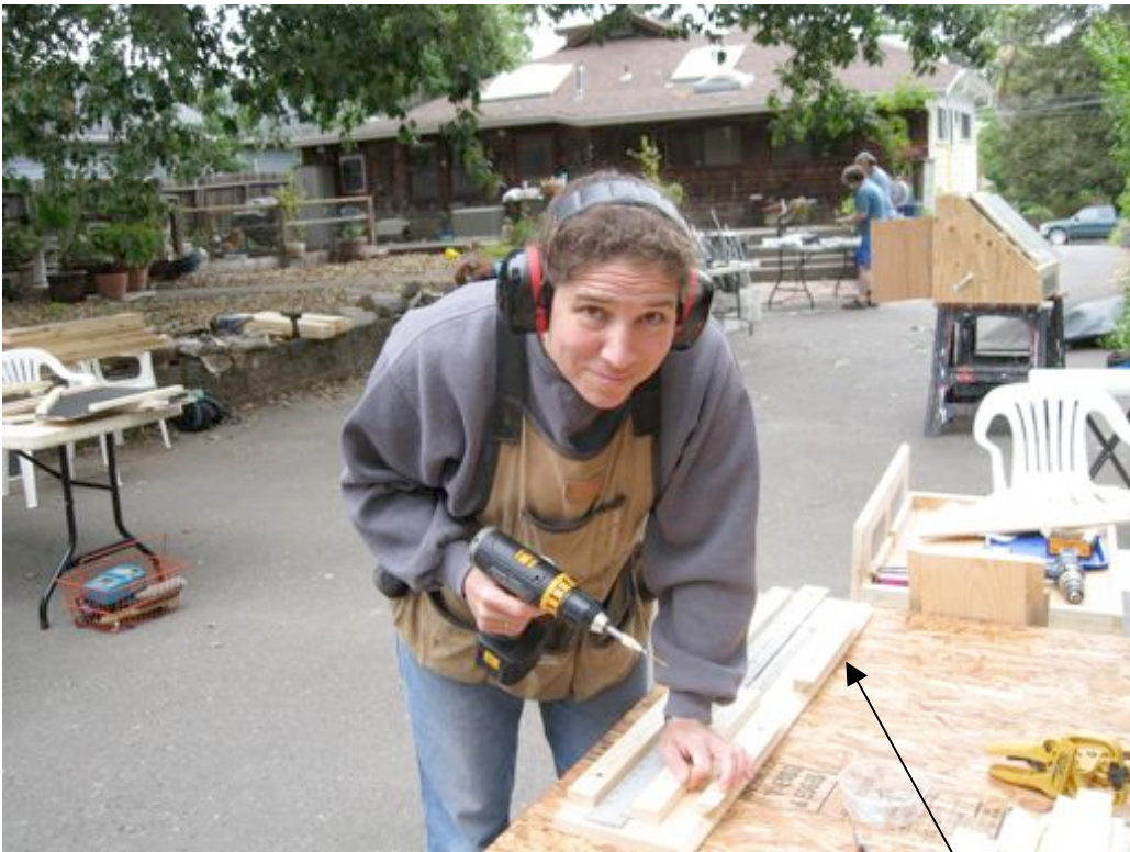
Attaching shelf supports to front board. Note the beveled plexiglass support.
