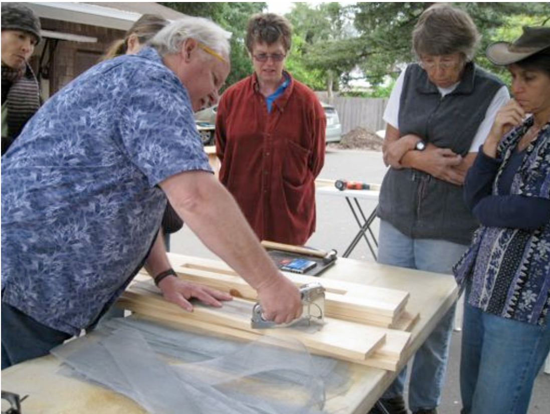
Attaching window screen (with edges folded over)...on inside of front and top/back boards...with folded side to board. Staples usually needed to be pounded in with a hammer after stapling.
